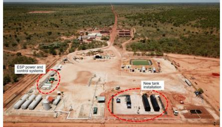
Ungani Production Facility showing ESP surface equipment and new tank installation
