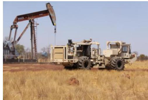
*Blina beam pump and seismic vibrator*
