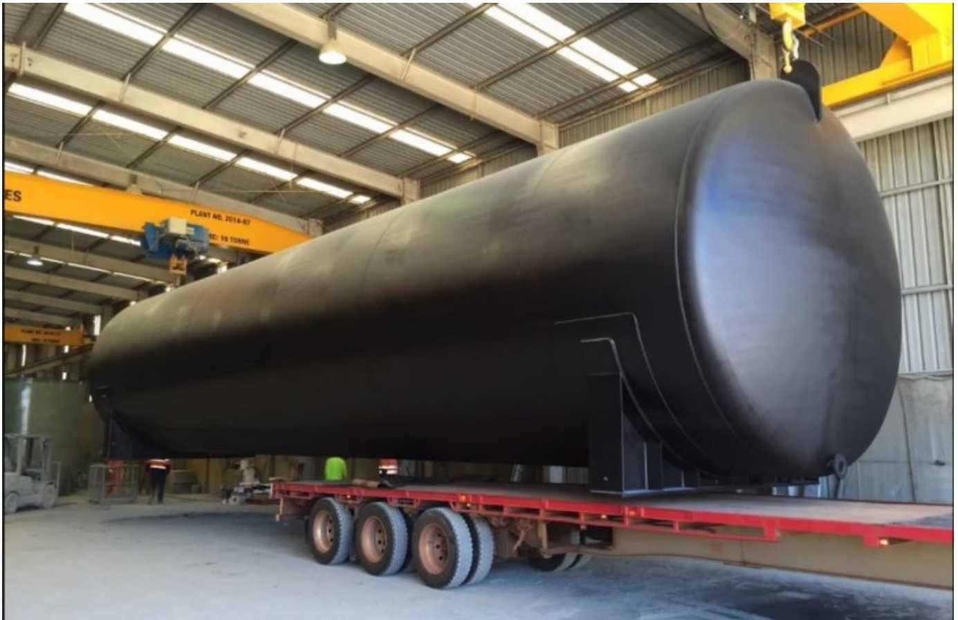
Buru's 1250bbl storage tank under construction.
