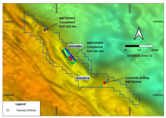
Figure 2: Locations of the drillholes at Barbwire Terrace over Bouguer gravity. Note the prominent gravity ridge (warmer colours) extending from the northwest to southeast, identifying the boundary between the Fitzroy Trough to the northeast, and the Barbwire Terrace to the southwest.
