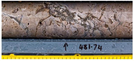
Figure 5: Brecciated carbonate and sulphides vein in dolomitised Pillara Limestone at 481.74m in hole BWTDD0003, with up to 1% Zn in spot pXRF readings. Core diameter is 47mm.
