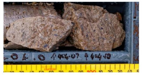
Figure 3: Disseminated galena in dolomitised Pillara Limestone at 404.07m in hole BWTDD0003, with 1.34% lead in spot pXRF reading. Core diameter is 47mm.
