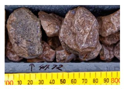
Figure 4: Disseminated galena in dolomitised Pillara Limestone at 411.72m in hole BWTDD0003, with 1% Zn and 3.1% lead in spot pXRF reading. Core diameter is 47mm.
