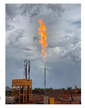
Once the cyclone conditions pass, the test will resume with a longer flow period and the acquisition of separator samples to determine more accurately the condensate and LPG content of the gas stream. A further update on flow rates and flow conditions will be provided at the conclusion of the test.
