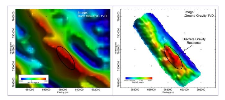
Gravity image from a portion of the Barbwire Terrace Project area showing the improved resolution of the ground gravity survey in the right-hand image compared with the Buru regional gravity image on the left. The 'discrete gravity response' in the right-hand image will be tested in planned drilling.
