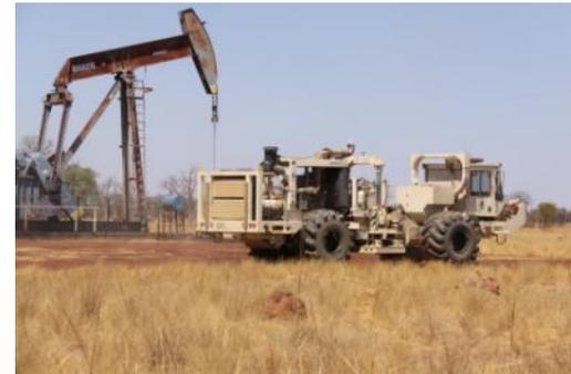
*Blina beam pump and seismic vibrator*
