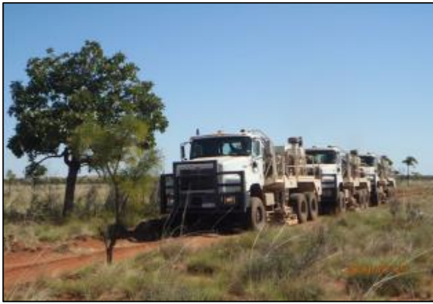
Seismic vibrators at Commodore West survey
