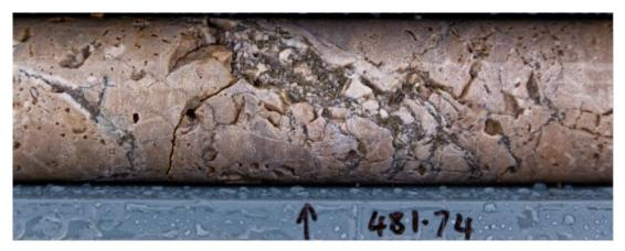
Figure 3: Brecciated carbonate and sulphides vein in dolomitised Pillara Limestone at 481.74m in hole BWTDD0003, with up to 1% Zn in spot pXRF readings. Core diameter is 47mm.
