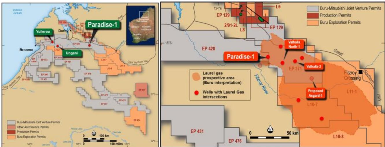
The existing Paradise-1 well was drilled by the Buru and Mitsubishi joint venture in late 2010 to a depth of 1,700 metres. The well was completed with 7" casing to that depth and then suspended due to operational issues and the onset of the wet season.
