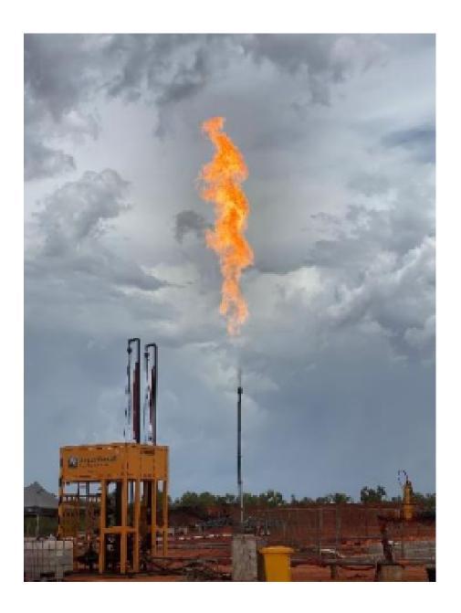
The indicative condensate gas ratio (CGR) was estimated to be between 20 to 30 barrels of condensate per million cubic feet of gas.
