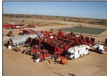
*Our Fracturing Locations will have a very similar setup to this location with a source water pit and 30,000 HHP of state of the art Fracturing Equipment. The equipment is controlled from inside of the "white Tech Command Centre" with real-time offsite monitoring of the job via Satellite communications.*
