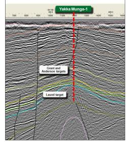
Seismic line showing Yakka Munga-1 location
