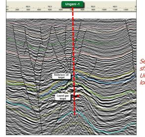
Seismic line showing Ungani-1 location
