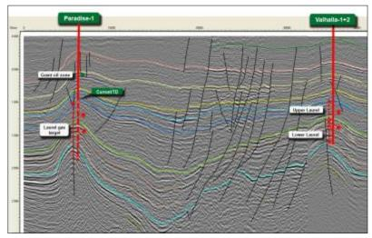
Seismic line showing Paradise-1 Deepening location and Valhalla structure
