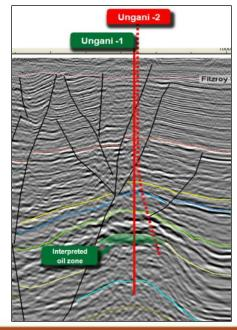
Seismic line showing Ungani-1 and 2 location
