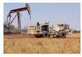
Blina beam pump and seismic vibrator
